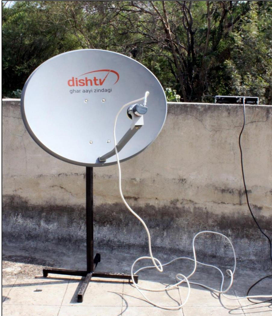
\* The pictures show the dish with the LNB Arm connected upside down. The LNB Arm should be connected such that the “UPSIDE” letters face up towards the sky after connecting it to the dish.
