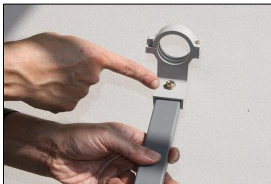
**Step 5:** Loosen the LNB Holder screw and insert the LNB with the Feed side facing towards the dish into it. Tighten the screw so that the LNB stays in place but allow for some slack so that the LNB can be rotated within the holder.
