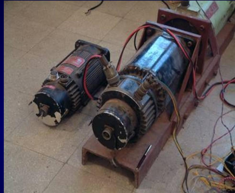
Pair of 6 HP DC servo motors in a counter-torque system for Azimuth and Elevation axes
