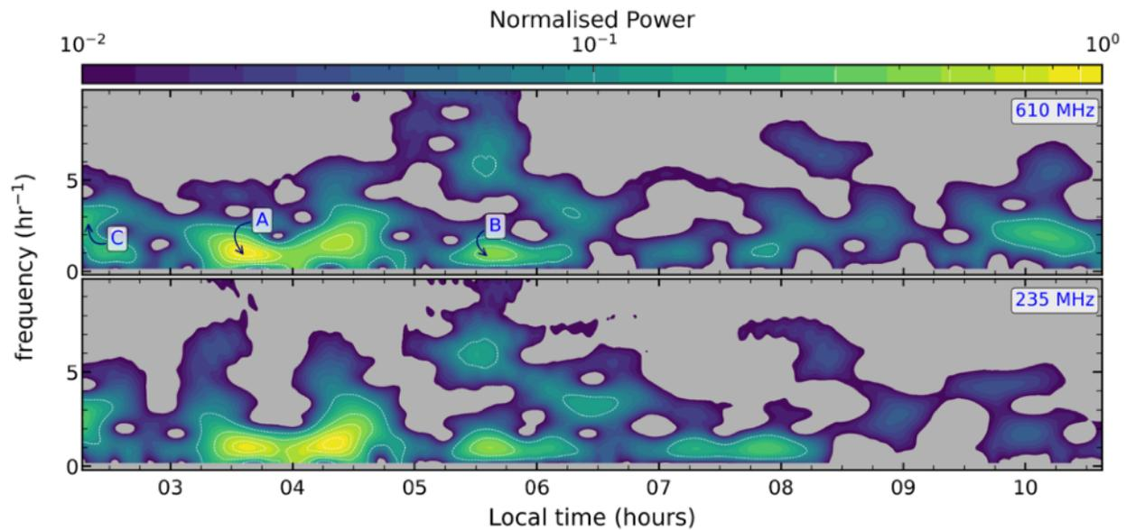
Figure 2: The normalized power as a function of temporal frequency (y-axis) and local time (x-axis). Similar structures are present in both bands, also, smaller structures are more visible in the 235 MHz band compared to the 610 MHz band.
