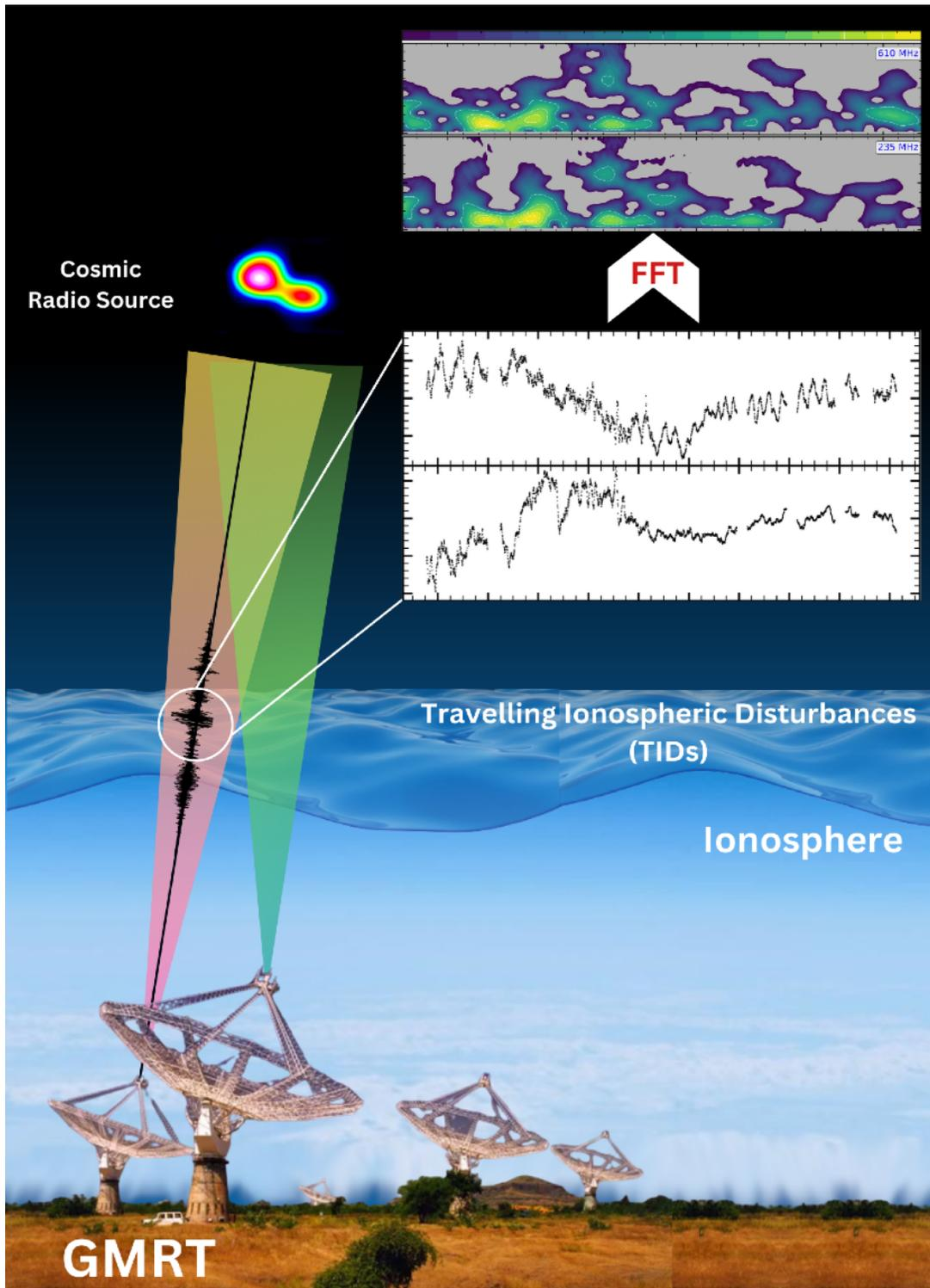
Figure 1: Illustration showing how ionosphere disturbs the distant signal receiving from radio sources and how GMRT detects these signals and better transform them into detecting ionosphere disturbances.
