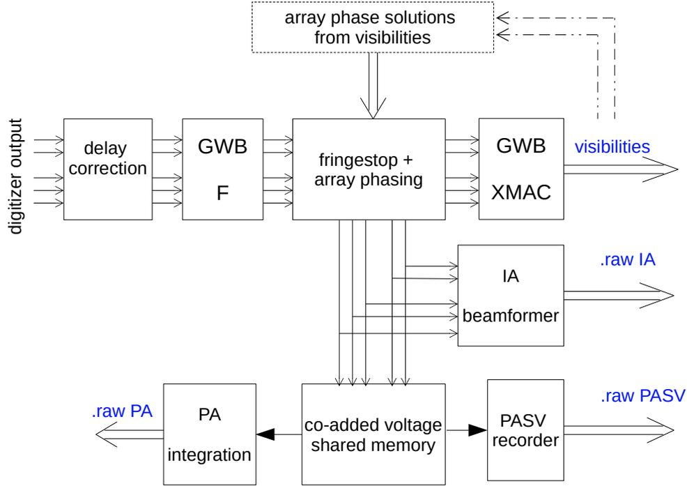
Figure 1: A high-level schematic view of the architecture of the GWB beamformer and the PASV block in relation to it. The CD pipeline is not shown here in the interest of clarity.
