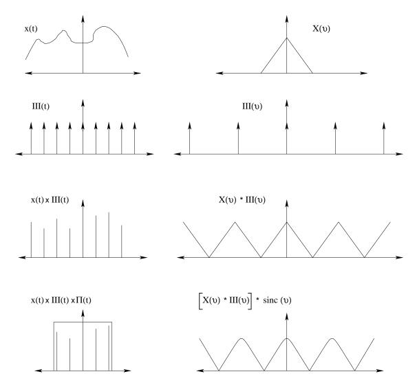
Figure 8.3: The relation between the continuous Fourier transform and the discrete Fourier transform. The panels on the left show the time domain signal and those on the right show the corresponding spectra.
