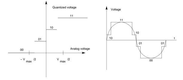
Figure 8.1: Transfer function of a two bit four level quantizer. The *binary* numbers corresponding to the quantized voltage range from 00 to 11. Quantization of a sine wave with such a quantizer is also shown.
