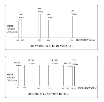
Figure 24.8: Schematic of the signals carried by the forward and return link. See the text for more information.
