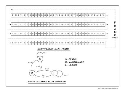
Figure 24.4: Structure of the multiplexed voice and data frame. Shown at the bottom of the figure is the flow diagram for the synchronous detector state machine.
