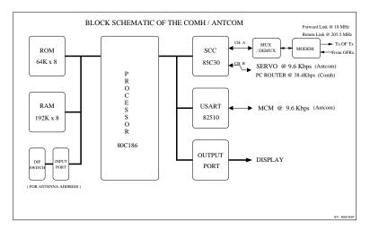
Figure 24.2: Block diagram of the GMRT communication handler (COMH). The antenna computer (ANTCOM) has essentially the configuration.
