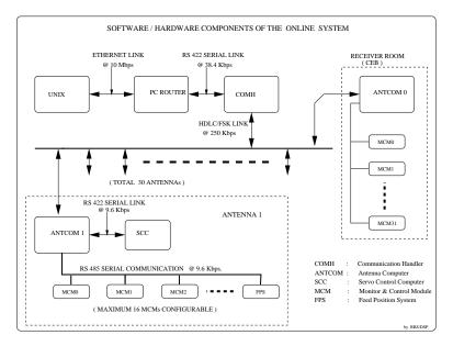
Figure 24.1: Block diagram of the GMRT monitor and control System. See the text for more information.
