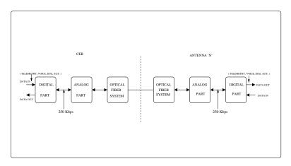
Figure 24.7: Schematic of the GMRT telemetry system. See the text for more information.
