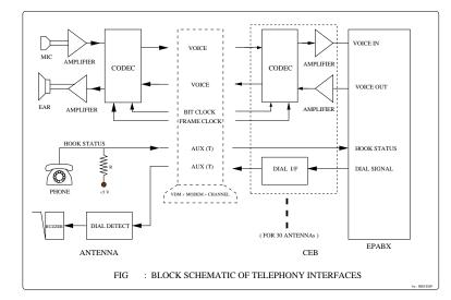
Figure 24.6: Block diagram of the telephony interfaces.
