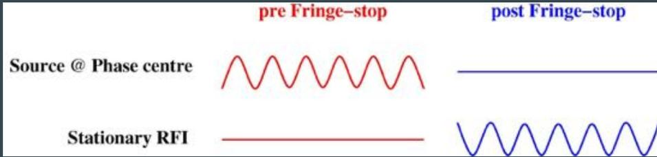
RFI causes the visibility vector to describe a circle as a function of time on the complex visibility plane.
